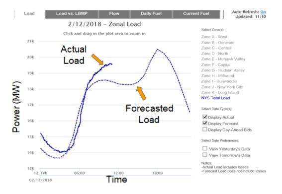
Figure 1.1.2: NYISO Load forecast (dotted) and actual load graph (solid) for 2/12/18. [1]
